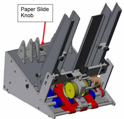
Figure III-9 Shrouded Separator
