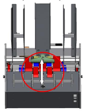
Figure III-3 Shrouded Separator
